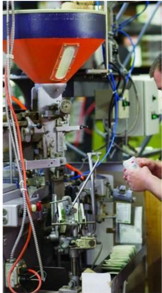
Seeds are poured into the red and blue hopper at the top. A set weight of seeds is let out of the bottom of the hopper. These are poured into the packet which is sealed and put into the tray. This picture was sent to me by Botanical Interests.
